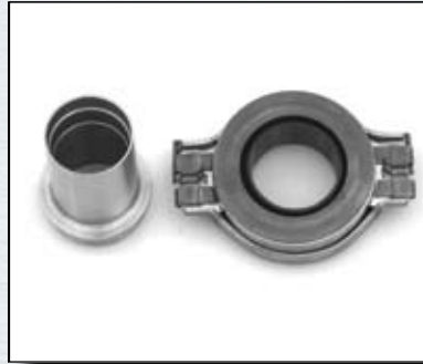
EARLY TO LATE T/O BEARING CONVERSION
